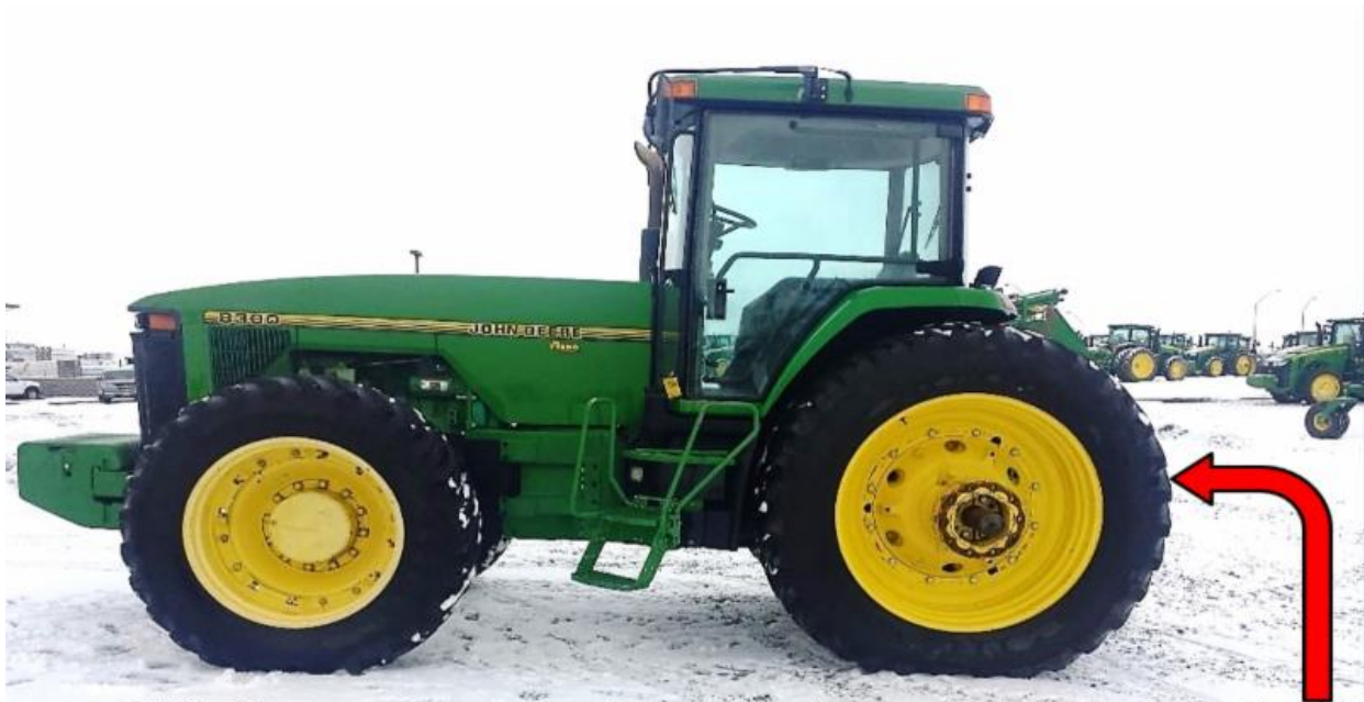
PIN Plate on transmission, above PTO output shaft
