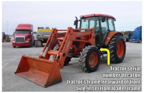
Note that the serial number decal on the left loader upright near the cab is only for the loader and does not identify the tractor. At the time of this alert, the loader model and serial number were not available to NER.
