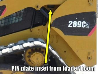
Closeup of the PIN location on a similar CAT Compact Tracked Loader (this is not the stolen machine).
