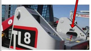
The machine serial number plate is on the right loader upright, above the engine compartment
