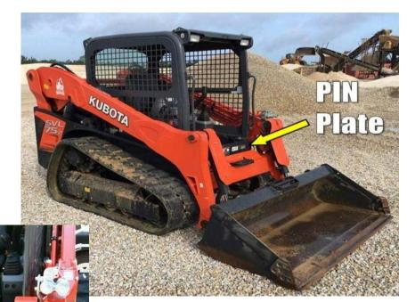
Within the cab is the ROPS serial number plate, which does not correspond to the machine PIN/Serial Number, and must not be confused as a machine identification.
