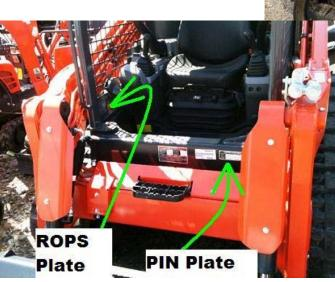
Within the cab is the ROPS serial number plate, which does not correspond to the machine PIN/Serial Number, and must not be confused as a machine identification.
