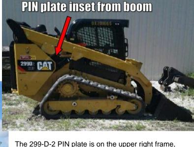
The 299-D-2 PIN plate is on the upper right frame, below the boom and rearward of the operator. The plate is obscured by the boom and hydraulic cylinder when the boom is in the lowered position.
