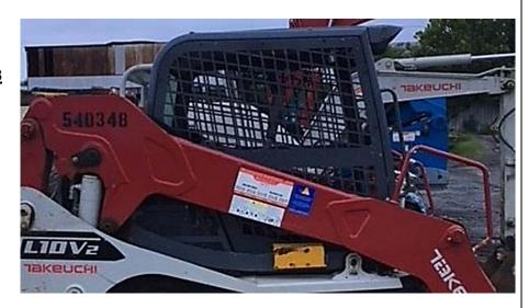
Pictured below is a similar TL-10 for illustration purposes. The machine serial number plate is on the right loader support structure, above the engine compartment.
