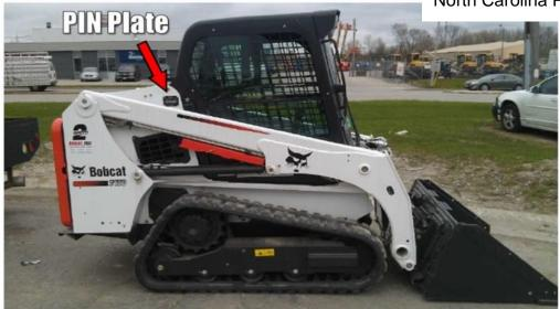
Pictured is an example of a similar Bobcat T-450. The machine PIN plate is on the right upper frame, just behind the cab and above the loader boom (with the bucket lowered).
