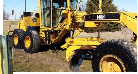
The below image is a similar CAT 140-H illustrating the PIN plate location on the left side of the goose-neck, forward of the cab.
