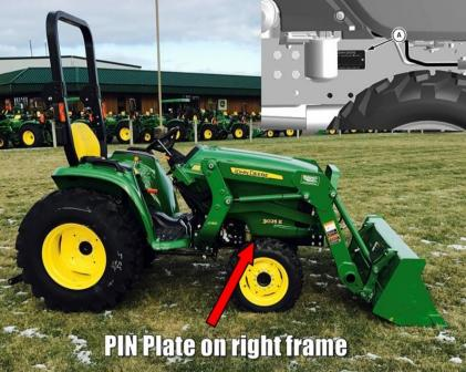
Pictured is an example image of a Deere 3025-E. The Tractor PIN plate is on the right frame, inset from the front wheel and partially obscured by the lower engine cover panel.
