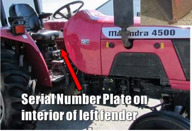
The Tractor Serial Number Plate is either on the dash or the left fender, next to the seat.
