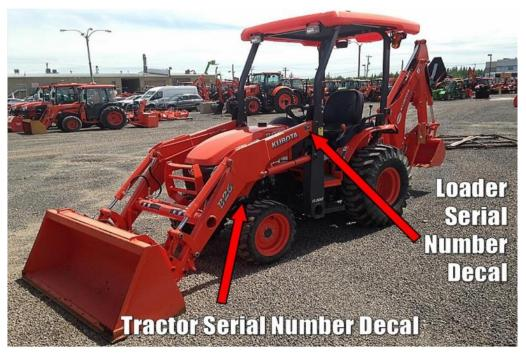
Pictured is an example of a similar Kubota B-26. The tractor serial number decal is on the left frame inset from the left front wheel. This must not be confused with the more prominent loader serial number decal on the left loader upright, which is only the loader identifier.
