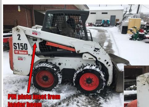
Pictured is another S-150 from the same fleet. Note the owner applied number "1" would appear the same as the number "2" does on the pictured machine. The machine PIN plate is above the right rear wheel, inset from the loader.
