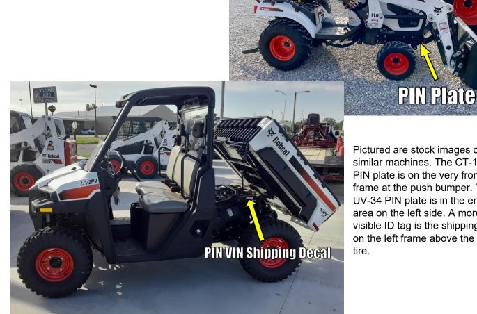
Pictured are stock images of similar machines. The CT-1021 PIN plate is on the very front right frame at the push bumper. The UV-34 PIN plate is in the engine area on the left side. A more visible ID tag is the shipping label on the left frame above the rear
